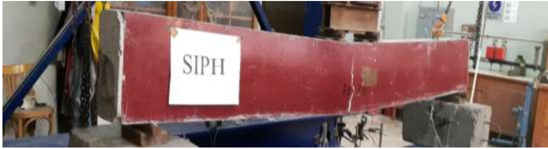
Figure.14. Failure mode of specimen (SIPH), (SIPHC) and (SIPHCI), the second mode.
