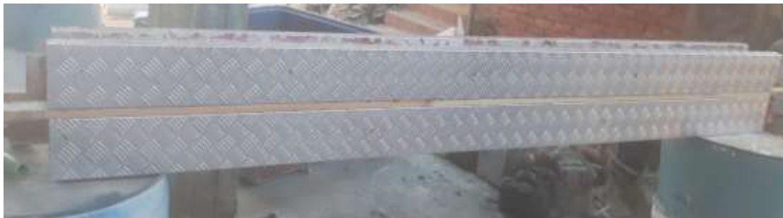
Figure. 2. Aluminum chequered plate mold for manufacturing of FRP forms.
